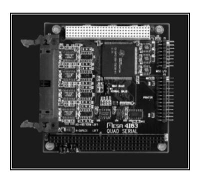
Since the 4I63 is a PCI card it has much lower overhead than ISA based serial cards and can support more channels at higher baud rates.
