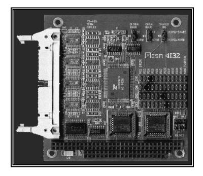
Each serial port can use any of the 11 available interrupts ISA bus interrupts. Shared interrupts are also supported, allowing the four per channel interrupts to be logically ORed to a single interrupt. The ORed interrupts are individually maskable, and the interrupt status of all four channels can be read at a single location. The receive and transmit FIFO status of all four channels can also be read at a single location.
