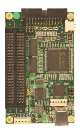
The I/O connectors are compatible with our 7 series daughter cards for isolated I/O, motion control and other applications.
