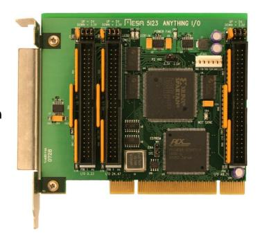
The MESA 5I23 is a general purpose programmable I/O card for the PCI bus. The 5I23 uses a 400 gate Xilinx FPGA for all logic, so it is truly an "Anything I/O" card.
