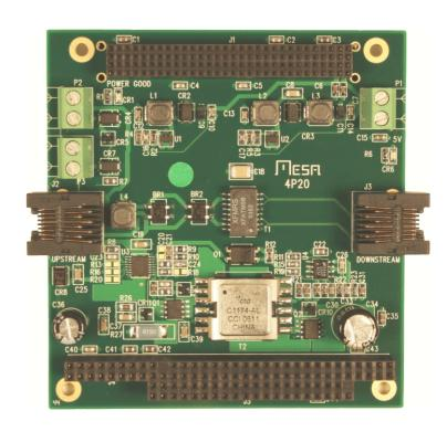
The 4P20 is a Power-Over-Ethernet power supply that allows remote operation of low power PC/104-PLUS stacks. The 4P20 provides a feed-through POE tap so that the remote system can get power and Ethernet communication from a single CAT5 cable up to 100 meters long. The 4P20 supplies 5V and limited amounts of +- 12V power to the stack. +-12 Volt outputs can be disabled if not required.
