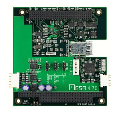
The 4I70 is a PC104-PCI remote cabled bridge. It allows expansion of PC/104-PCI systems via a serial data cable up to 30 feet long. The 4I70 appears to the system to be a standard PCI bridge so no special software or drivers are required for use. The 4I70 can be jumpered for forward (cable to PCI master) or reverse (PCI slave to cable) mode. When in forward mode, the 4I70 replaces the CPU in a PC/104-PCI stack, supporting up to 4 bus master peripheral cards.
