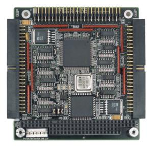
The 4l36 counters can count in normal quadrature mode (4X) or up/down mode (1X). Digital filtering is used on encoder inputs to reject input noise. Each counter has a option to be cleared by either the rising or falling edge of the index signal.
