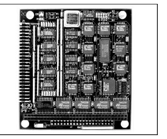
The MESA 4I30 is a stackable PC/104 card with four 32 bit up/down counters with quadrature count inputs and per channel index inputs. The 4I30 is intended for robotic, motor control, measurement, and instrumentation applications.
