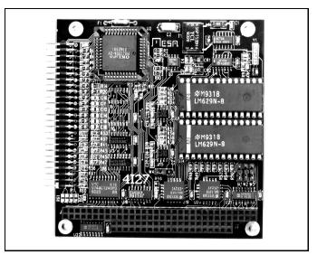
The 4l27 is a low cost, LM629 based 2 axis DC servo motor control system implemented on a stackable PC/104 bus card. The 4l27 is designed for high performance positioning systems using DC servo motors with quadrature shaft encoders. The per axis output of the 4l27 is an 8 bit sign-magnitude PWM signal that can drive H-bridge type servo amplifiers directly.
