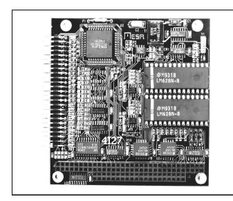
The 4I27A is a low cost, LM628 based 2 axis DC servo motor control system implemented on a stackable PC/104 bus card. The 4I27A is designed for high performance positioning systems using DC servo motors with quadrature shaft encoders and analog input servo amplifiers.
