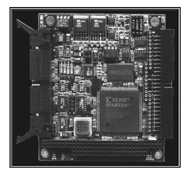
The conversion start timer is a 24 bit, 50 MHz programmable divider for high resolution and wide conversion rate range.
