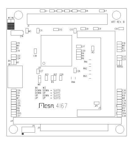
The 4I67 is a PC/104-PLUS to dual Mini-PCI III adapter. The 4I67 allows two Mini PCI type III cards to be connected to a PC/104-PLUS system. Since the 4I67 uses a PCI-PCI bridge, it only uses one PC/104-PLUS slot.
