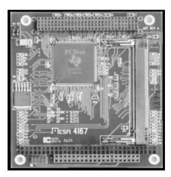
The 4I67 is a dual type III Mini-PCI adapter for the PC/104-PLUS bus The 4I67 allows use of 2 Mini-PCI cards like IEEE 802.11 wireless LAN cards in a PC/104-PLUS system.
